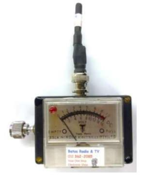
Rf sniffer is a Simple (no batteries required) Field Strength Meter yet also quite sensitive . It has sensitivity adjustment.
